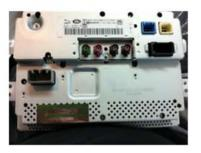
Place of installation is at the back side of the monitor.
