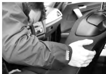
N°6. Move the seat to the front to have access to rear screws
