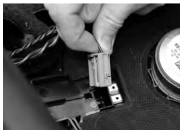
N°17. Disconnect the factory plug to terminal
