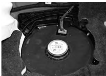
N°16. Subwoofer is accessible and be removed
