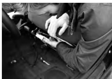
N°8. After 4 screw unscrewed, fall over the seat to the front position
