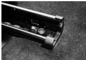
N°2. "Front" screws to remove the seat
