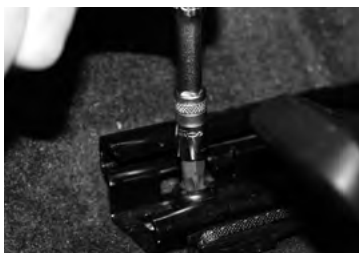
N°5. Unscrew with a "torx 45" tool
