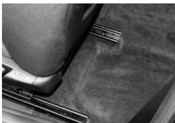
N°3. "Rear" screws to remove the seat
