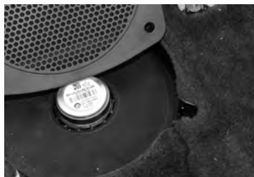
N°14. The BMW factory subwoofer is under the grille
