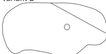
2. Install the KCX802-ECO on the back of your car for instance. Drill a hole of 8mm.
