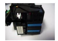
Insert the Connects2 lead into the empty slot:
