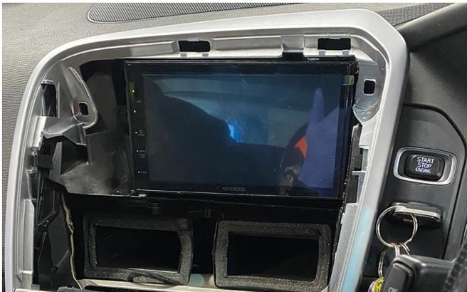
With the brackets affixed to the correct sides of the stereo and the dashboard modified, connect up the stereo and slot into place, screwing into place using the pre-existing screws.
