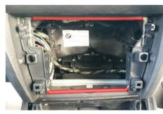
4. Cut inside the dash trim along the two lines at the top and bottom as highlighted.
