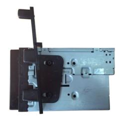
6. Screw the supplied plastic brackets to the side of the aftermarket head unit. The mounting depth can be adjusted accordingly via the mounting holes.
