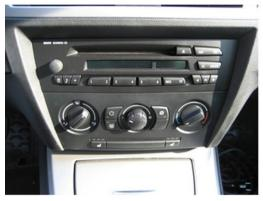
Remove the climate control panel using a panel removal tool.
