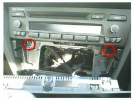
2. Unscrew the two screws holding the OEM radio in place. Slide the radio forward and disconnect
