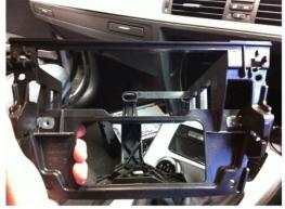
3. Unscrew the plastic sub-dash cage and remove from the dash.
