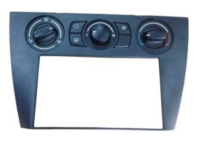
5. Remove the climate control panel from the OEM climate control bezel. Insert this into the panel supplied in the CT23BM08 kit.
