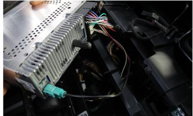
9. Reroute the four (4) connections from the air conditioning panel up and out on the right hand side of the top dash tray
