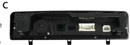
12. Connect the included extension leads to the back of the button relocation panel, and the preexisting connections of the vehicle (removed in Step 6)
