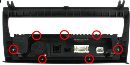
11b. Place the button panel inside the included trim as shown in Fig.b
