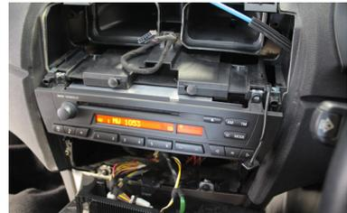
6. Disconnect the four (4) connections to the air conditioning panel
