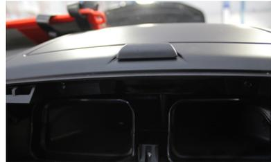
5. Use a Panel Removal Tool to remove the air conditioning panel and trim
