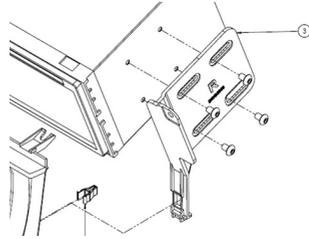
14. Place the stereo and bracket assembly into the dashboard, making all wiring connections, and screw into place using the OEM screws
