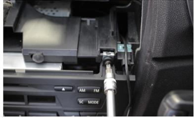
8. Remove the OEM radio and disconnect the DAB antenna (if vehicle is equipped) and quadlock connector
