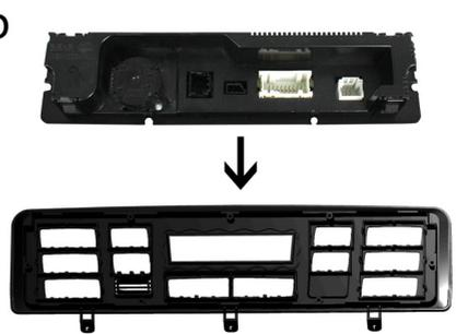
11c. Use the screws removed in Step 11a to reattach the button panel to the included trim piece, creating the new climate control button assembly for use in the installation.
