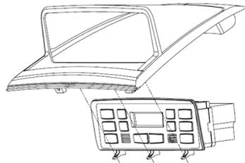
17. Finally reconnect the hazard switch, pushing it into place, to complete the installation.
