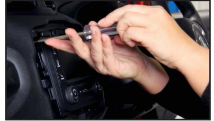
With the main fascia panel out of the way, undo the following four screws and put these to one side. With the screws out, fully remove the head unit whilst disconnecting all of the wiring.
