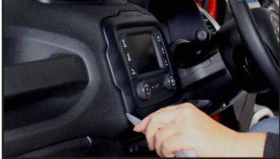
Using a panel removal tool, begin to unclip the main fascia panel that sits around the main head unit.
