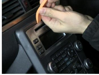
2. Removing the panel will reveal 2 long screws located at the top of the main fascia panel. You will then find a further 4 screws toward the arm rest as well as behind the fascia panel that will need to be removed.
