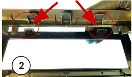
**2.** due to varying thicknesses of OEM dashboards some vehicles may need the area **circled** filing to make the clips locate and lock correctly.
