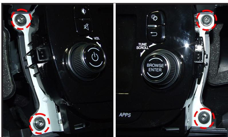
When the main fascia trim has been removed, undo the 4x screws found on either side of the main unit and proceed to pull it out of the dash whilst disconnecting all of the wiring.
