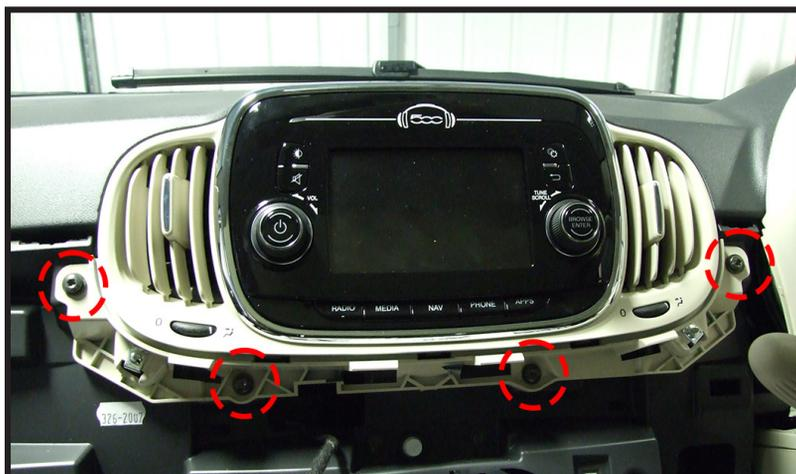
With the dashboard trim panel out of the way, proceed to undo the 4x highlighted torx screws that surround the main fascia trim. Once free, pull upwards away from the dash.
