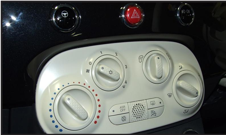
To begin, use a panel removal tool to unclip the climate control button panel. Be careful not to damage the surrounding trim.
