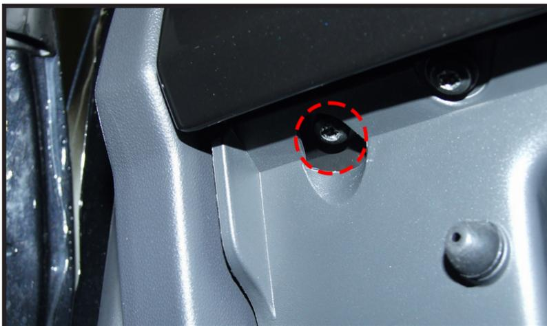
Now open the glovebox, within the lip on the far side nearest to the passenger side door will be a recessed torx screw. Once this screw has been undone, proceed to fully remove the dashboard trim by means of a panel removal tool, disconnecting the button panel in the process.
