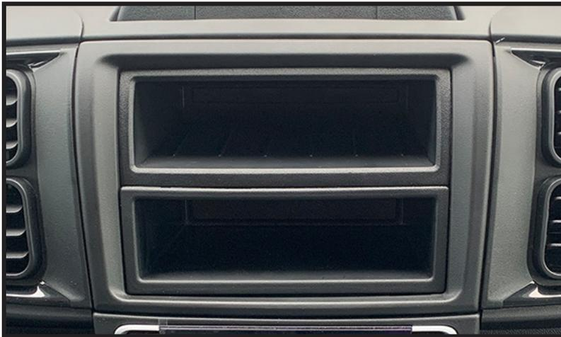
Begin by using a panel removal tool to unclip the two pockets that sit where the main head unit would normally sit.
