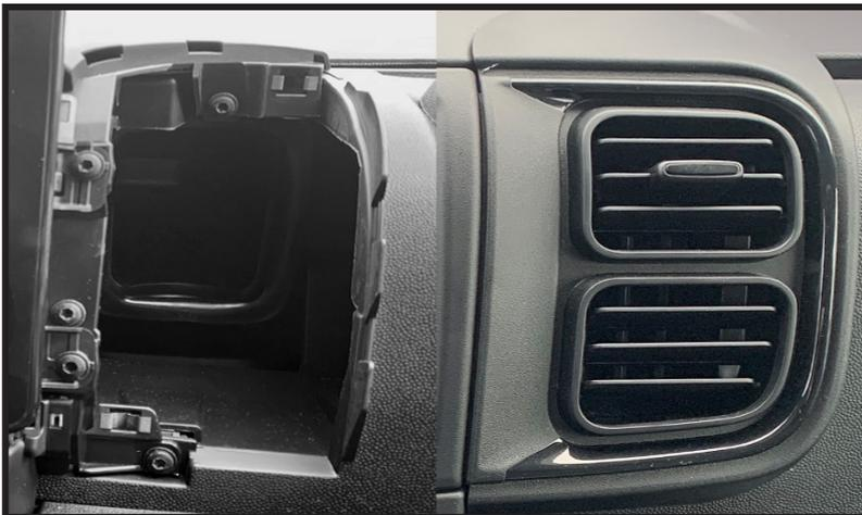
Use the panel removal tool to unclip the entirety of the side air vents. Once free, simply pull them out of the dashboard and set them to one side.
