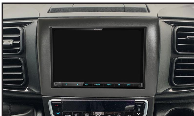
With the cage in place, and the head unit connected correctly, proceed to slot the radio into the dashboard until it clips into place. Carry on to finish the installation by placing the trim around the head unit and re-assembling the dashboard in reverse order.
