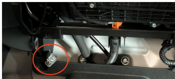
5. Route the pin end of the speed/reverse wires from the main dash aperture through and down toward the fuse panel. The bare ended wires will remain in the dashboard aperture for use on the new head unit.
