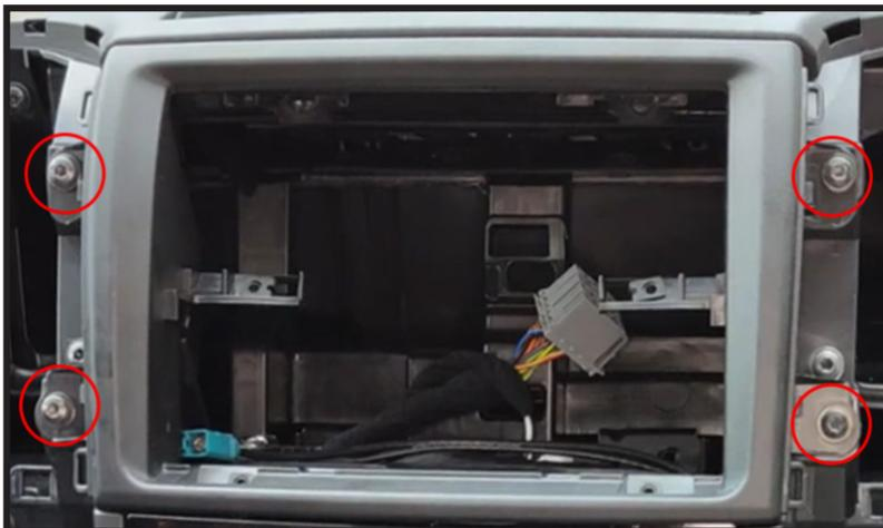
With the air vents removed, you will then need to undo the 4x screws that surround the main fascia. Once undone, simply pull the fascia away from the dashboard.
