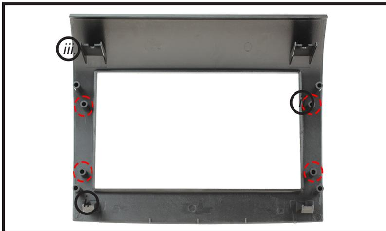
Using the 4x phillips screws, take the brackets and line them up to the following posts on the rear of the new fascia panel and proceed to attach them to the relevant side.
