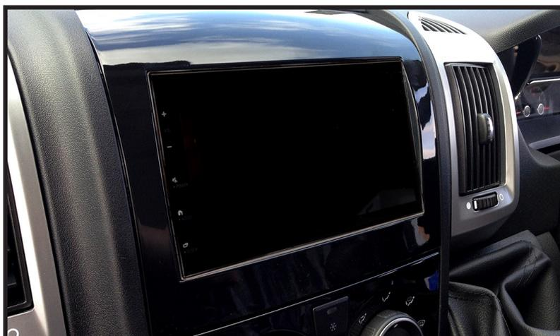
Once the kit has been assembled and the wiring for the stereo is completed, simply use the clips within the kit on the reverse of the fascia and proceed to clip it into place.
