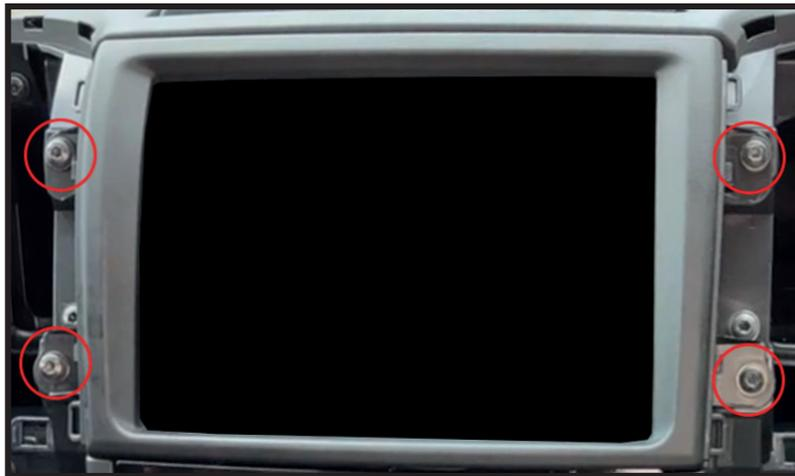
With the air vents removed, undo the 4x screws that surround the main head unit. Once undone, simply pull the fascia away from the dashboard and disconnect all of the wiring.
