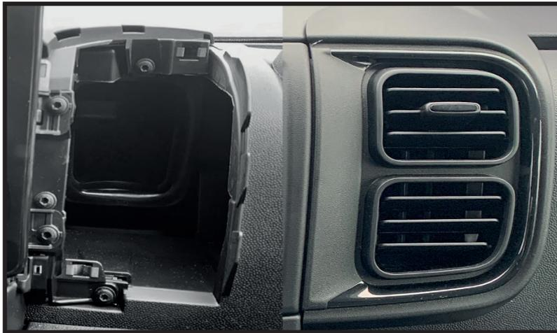
Begin by using a panel removal tool to unclip the entirety of the side air vents. Once free, simply pull them out of the dashboard and set them to one side.
