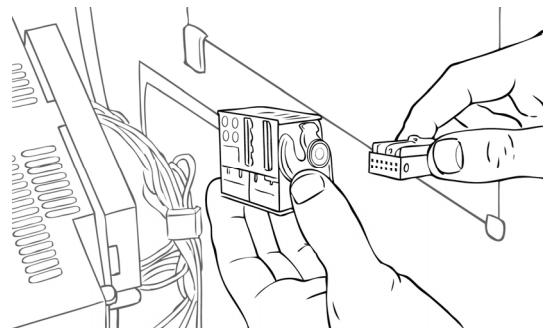
In some cases there may be an add-in connector. Remove the CD changer section and replace with the loom supplied with the Gateway Lite. Turn page over for car-specific connections.
