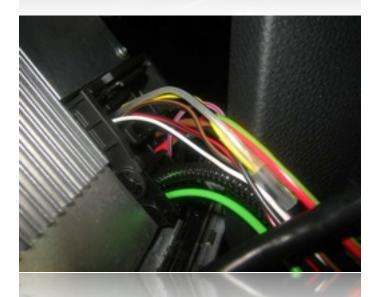
Unplug the connector from the back of the drive unit and set aside.
