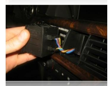
Like so. Disconnect and set aside, then fully remove the dash trim as described above and set aside.
