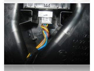
Now, the connector that plugs into the door lock and DSC switch mounted in the middle of this trimpiece must be disconnected. This is easily done by following the steps below.
