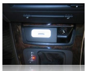
After removing the backing from the double-sided tape on the bottom side of the dock and lowering the spec.dock into position, the console may be reinstalled to finish the electrical portion of the installation. Be sure to verify all connections and functionality before completely reassembling the vehicle, but again **do not turn on the vehicle ignition until all unplugged connectors are reassembled.** Reassembly of the vehicle is the opposite of disassembly.
