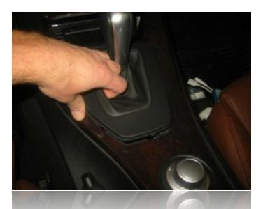
Begin by unsnapping the shifter trim with your fingers. Pulling gently will be sufficient to release the clips that hold this piece in place.
