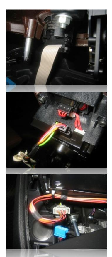
Underneath this trim are three connectors that will need to be unplugged to remove it completely from the vehicle.
