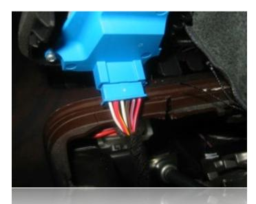
And this one. Unplug both. Once these connectors have been unplugged, do not turn the vehicle's ignition on until all connectors have been reassembled.
