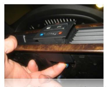
Reach behind the switch and push forward to unsnap it from the trim. Slide the switch out to gain access to the connector.
