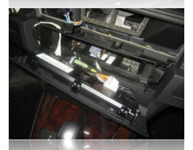
Unplug all the connectors on the back of the climate controls and set aside.
