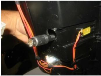
Route the wiring from the spec.dock through this hole and toward your audio connection point, which will differ depending on the interface option you chose. Please refer to the manual that came with the interface for connection details.
