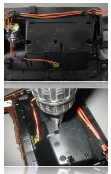
Now that the center console trim and ashtray assembly are removed from the vehicle, use a step drill bit to drill a 1/4" pilot hole in the location shown, then enlarge this hole to allow the cable emanating from the spec.dock to pass through.
