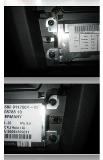
Remove the four Philips-head screws shown on the CD/DVD drive unit.
