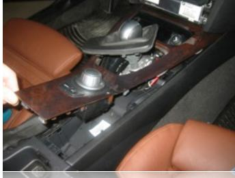
Use a panel tool such as the one shown to begin unsnapping the console trim, again being very careful not to chip the finish on the trim.
