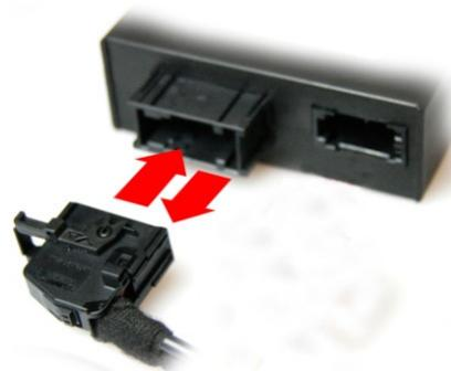
After restarting the optical circle the **Power supply** of the interface has to be **disconnected** and connected again.
